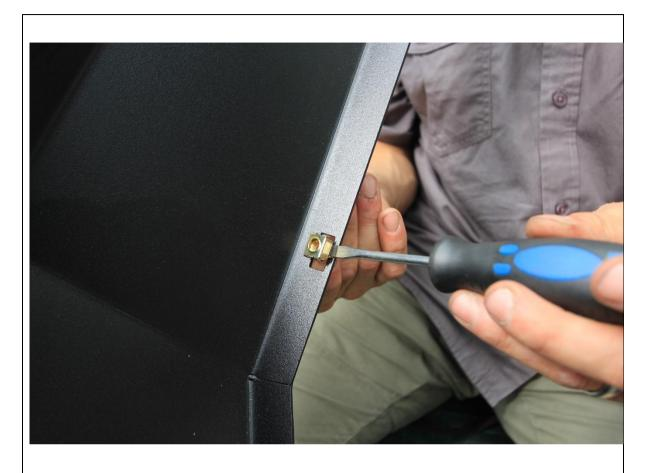
89. Insert cage nuts to square slots in bottom of wings, 3x per side. Seat cage nut against one edge of slot then, push other edge in with flat bladed screwdriver.
