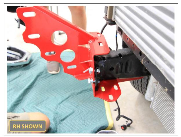
69. Fit front impact absorber mount assembly to the chassis.
