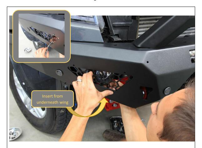
139. Fit light mesh panels to the bar. Position the panel from underneath the bar and align with the mounting holes in the wing. Secure with 4x M6x16 black button head bolts and flange nuts (no washers).
